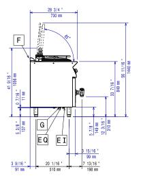
Cold Water inlet 1 (cleaning) HWI = Hot water inlet D Drain
